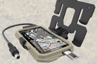
Connectorized Kägwerks EUD case
