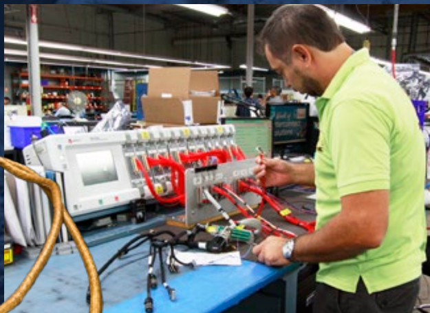
Continuity testing standard on all cable circuits
