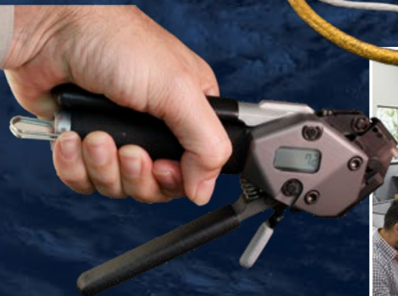
Reliable Band-Master ATS® EMI/RFI shield termination technology used extensively throughout the shop
