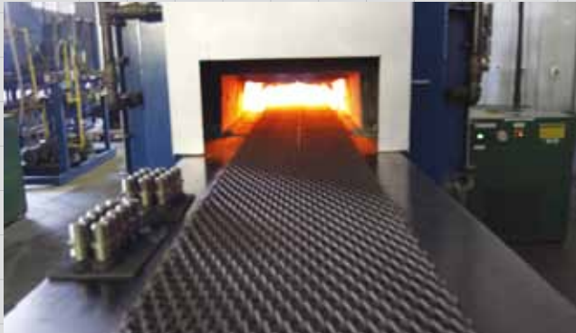
The connectors enter the furnace on a conveyor belt and a gas-tight hermetic seal is formed around all contacts, and between the glass seal and the connector shell, when the vitreous glass is melted in the furnace and then cooled under controlled conditions.
