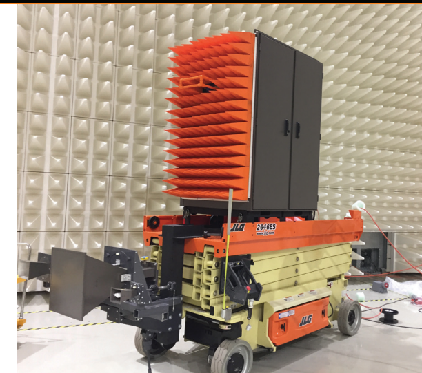
Customized system designed to address EUT height test requirement.
