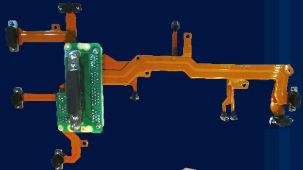
Hybrid flex/rigid multibranch assembly ready for connector termination
