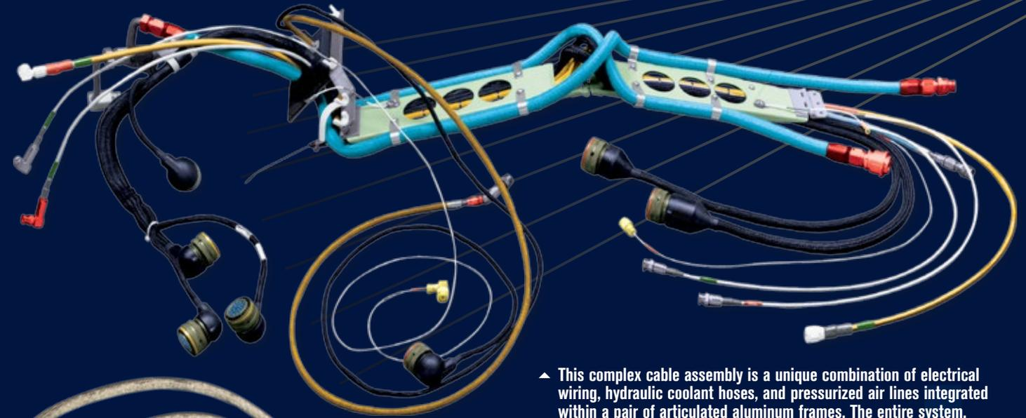
▲ This complex cable assembly is a unique combination of electrical wiring, hydraulic coolant hoses, and pressurized air lines integrated within a pair of articulated aluminum frames. The entire system, including coolant hoses, is assembled and tested according to customer specifications.
