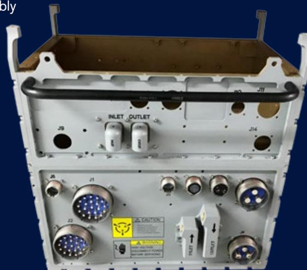
Fully connectorized and wired power console
