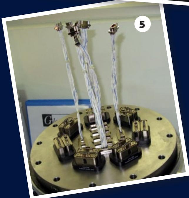
**Integrated Systems:** all interconnect components, boxes and machined chassis manufactured by Glenair. All cabling and final integration completed by Glenair. Glenair engineering provides extensive design support throughout.
