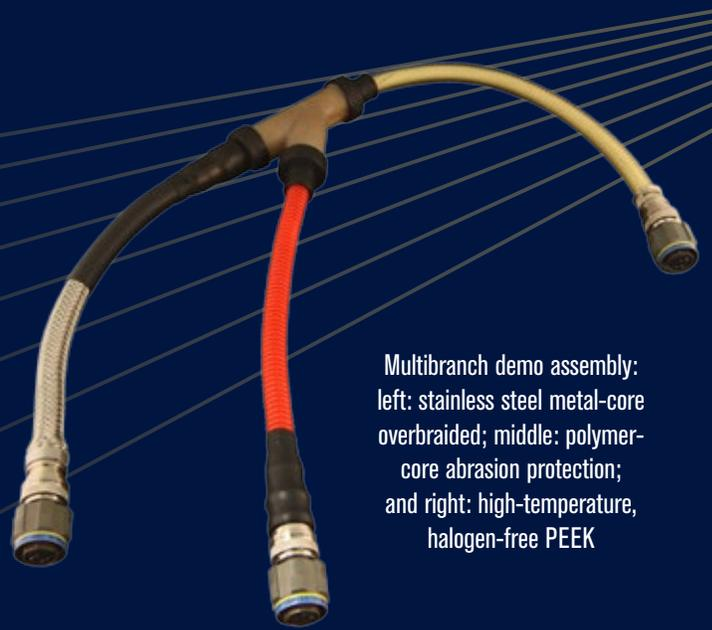
Multibranch demo assembly: left: stainless steel metal-core overbraided; middle: polymer-core abrasion protection; and right: high-temperature, halogen-free PEEK
