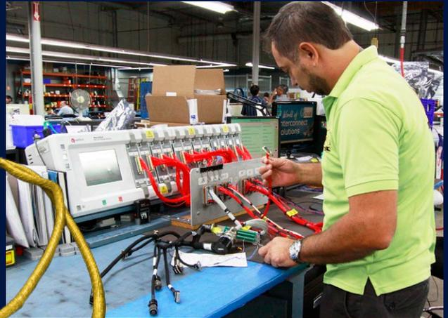
▶ Continuity testing standard on all cable circuits
