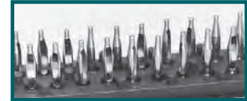
“Bi-Spring” Termination utilized on signal contacts
