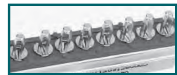
“Bi-Spring” Termination utilized on signal contacts
