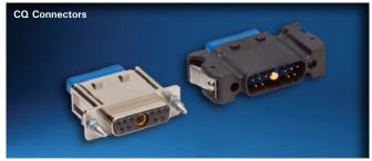
The CQ connector's unique design emits an audible click when mated. It is ideal for blind mating applications and hard-to-reach places, such as under passenger seats. It mates with any standard D-Subminiature or MIL-C-24308 connector, when lockpost hardware is installed.
