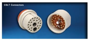
The CSLT is a quick coupling connector which can be used with PC tail and solder cup contacts in the receptacle and standard AS39029 size 20 contacts in the plug. Also this connector can be polarized in six different positions. The bayonet post design on this quick coupling connector is just an example of the capabilities we have available for your custom interconnect solutions.
