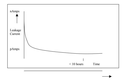
Good devices stabilise out very quickly – poor devices frequently show an increase in leakage or do not stabilise at all.
