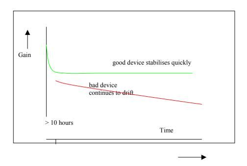
These examples relate to a single transistor. In Integrated circuits, the same actions take place except that on several hundred devices (in a simple IC) through to a few million devices (complex circuit). Drift of characteristic within and IC usually means that it will cease to function after a while (usually within the first 10 hours under stress).
