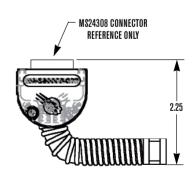
**NOTES** 1. THE PARTS SHOWN IN THE ABOVE TABLE ARE DESIGNED FOR M24308 CONNECTOR TYPE WITH STANDARD DENSITY OF 15 POSITIONS AND HIGH DENSITY OF 26 POSITIONS. OTHER SHELL SIZES, STRAIN RELIEF DIAMETERS AND DIFFERENT LENGTHS OF CONVOLUTED TUBES WILL BE AVAILABLE UPON REQUEST. 2. PARTS ARE PACKAGED UNASSEMBLED.
