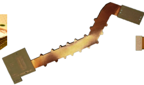
▲ Complimentary quick-turn mockups produced by by Glenair: 28-layer rigid flex (close-up and full-length), and 12-layer multibranch rigid flex
