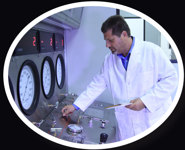
5. Small connector pressure test bunker
