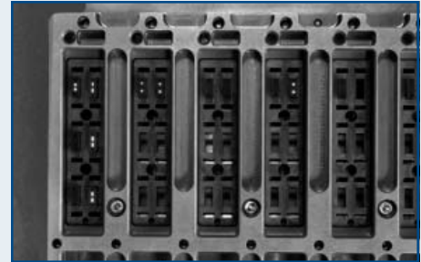
MT Ferrule Optics in Backplane Systems
