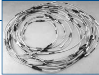
ARINC 629 Cable with Cable Couplers
