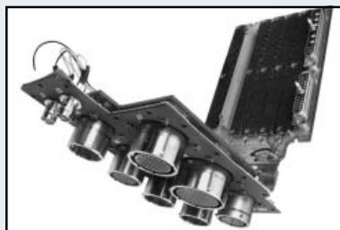
Backplane with MIL-DTL-38999 Cylindrical Connectors
