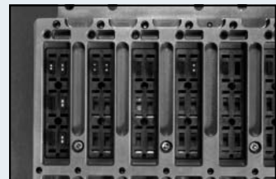
Backplane with MT Optical Ferrules
