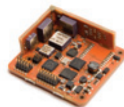
OEM: 37x33x12 mm, 11g 24-pins header
